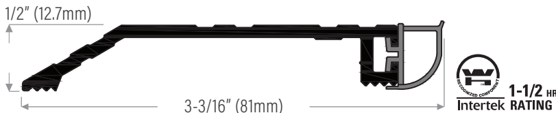
DS333AV Extruded aluminum mill finish with vinyl insert, grey DS333DV Bronze anodized
