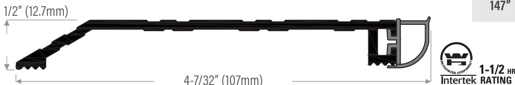
DS444AV Extruded aluminum mill finish with vinyl insert, grey DS444DV Bronze anodized
