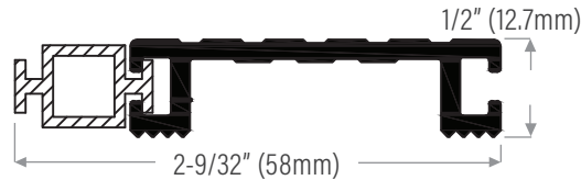
DS202TBA Extruded aluminum mill finish with thermal break insert
