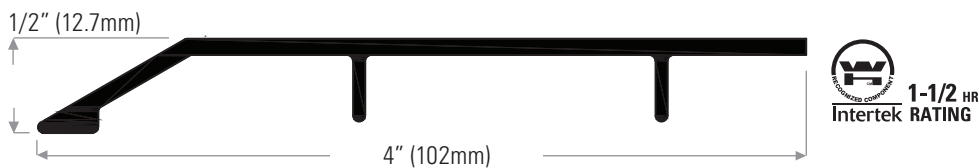
DS444AS Extruded aluminum mill finish
