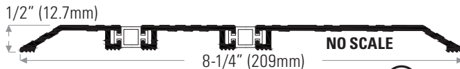
DS804TBA Extruded aluminum mill finish with 2 thermal breaks, 8-1/4" (209mm) wide DS804TBD Bronze anodized
