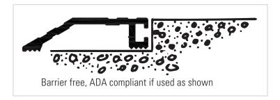
DS444 is supplied with punched countersunk holes with screws and plugs and is only available in the following NET lengths: 36-1/2" (927mm), 49" (1245mm), 73" (1854mm), 110" (2794mm) & 147" (3734mm)
