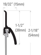
**DS162AV** Extruded aluminum mill finish with vinyl insert, grey.
