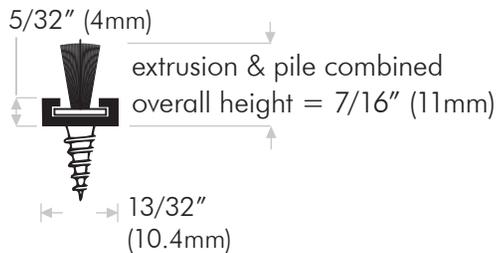
**DS369A7540G** Aluminum extrusion mill finish with fin pile insert, grey
