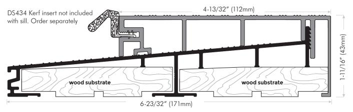
**DS657AVW** Extruded aluminum sill, mill finish with interior fixed vinyl top, white **DS657AVT** Extruded aluminum sill, mill finish with interior fixed vinyl top, tan **DS657AVBL** Extruded aluminum sill, mill finish with interior fixed vinyl top, black
