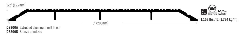
Thresholds are supplied with punched countersunk holes with screws and plugs and are only available in the following NET lengths: 36-1/2" (927mm), 49" (1245mm), 73" (1854mm), 110" (2794mm), 147" (3734mm)
