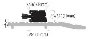
**DS176AP** Extruded aluminum mill finish with pile insert, grey, **not rated.** Threshold not included, order separately
