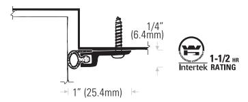
**DS103AT** Extruded aluminum mill finish with TPE (T) insert
