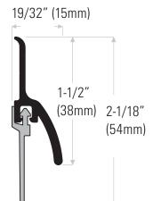
**DS162AV** Extruded aluminum mill finish with vinyl insert, grey. **DS162DV** Bronze anodized
