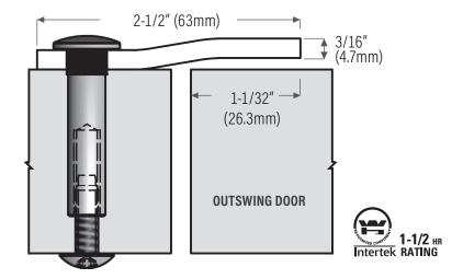
**DS179PS** Steel prime coated, pre-drilled
