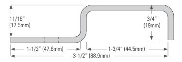
DS186PS Steel prime coated, custom. Lengths available 84" (2134mm), 96" (2438mm) & 120" (3048mm)
