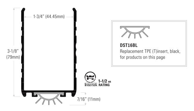
**DS212AT** Extruded aluminum mill finish with TPE (T) insert **DS212DT** Bronze anodized
