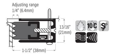
**DS340CN** Extruded aluminum clear anodized with neoprene insert, black **DS340DN** Bronze anodized. Custom order, call for manufacturing time.
