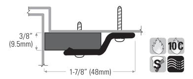
**DS131CN** Extruded aluminum clear anodized with 3/8" x 1-1/4" (9.5mm x 32mm) neoprene insert **DSN31BL** Replacement neoprene insert, black
