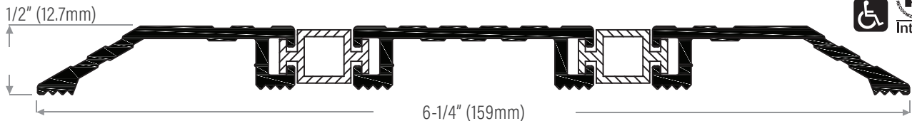
DS603TBA Extruded aluminum mill finish with 2 thermal breaks
