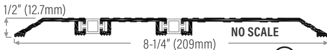
DS804TBA Extruded aluminum mill finish with 2 thermal breaks, 8-1/4" (209mm) wide DS804TBD Bronze anodized
