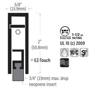
**223NA** Extruded aluminum clear anodized with neoprene insert, black **223NDKB** Bronze anodized with neoprene insert, black. Custom order, call for manufacturing time. 36" & 48" only (914mm & 1219mm)
