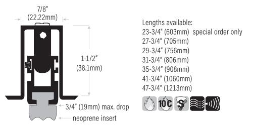
**423N** Extruded aluminum mill finish with neoprene insert, black. Available with lead insert for radiation shield. Specify "lead lined" custom order, call for manufacturing time.
