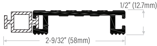
DS202TBAN Extruded aluminum mill finish or black anodized with thermal break insert
