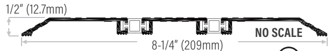
DS803TBA Extruded aluminum mill finish or black anodized with 2 thermal breaks, 8-1/4" (209mm) wide
