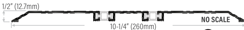
DS1003TBA Extruded aluminum mill finish or black anodized with 2 thermal breaks, 10-1/4" (260mm) wide
