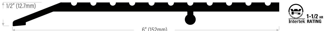
DS666HA Extruded aluminum heavy duty, mill finish or black anodized
