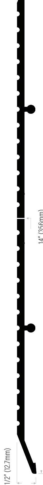
DS1400HA (2 piece) extruded aluminum mill finish, not welded
