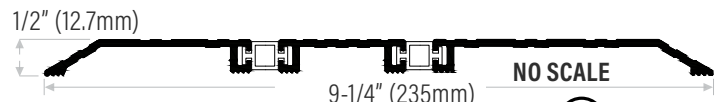
DS903TBA Extruded aluminum mill finish or black anodized with 2 thermal breaks, 9-1/4" (235mm) wide
