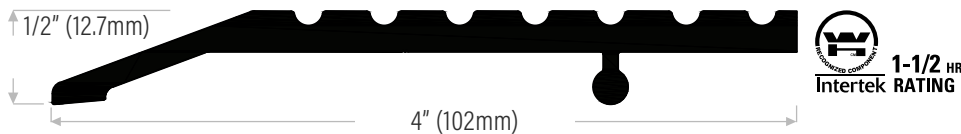
DS444HA Extruded aluminum heavy duty, mill finish or black anodized
