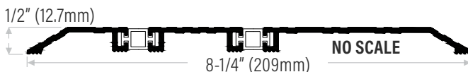
DS804TBA Extruded aluminum mill finish with 2 thermal breaks, 8-1/4" (209mm) wide DS804TBD Black anodized
