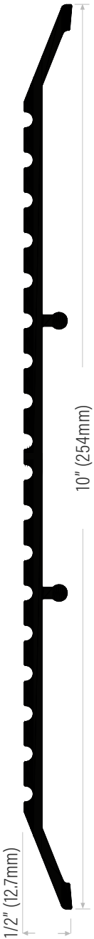
DS1000HA (1 piece) extruded aluminum mill finish DS1000HD (1 piece) bronze anodized
