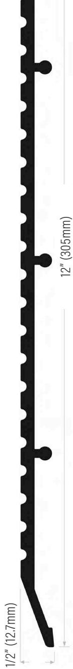
DS1200HC (1 piece) extruded aluminum clear anodized
